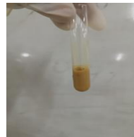
Figure 2; Positive 1% lead acetate test
