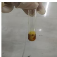
Figure 1; Positive 10% lead acetate test
